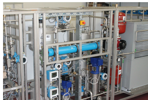
Reverse osmosis for seawater desalination
